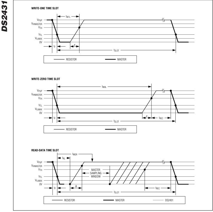
Figure 11. Read/Write Timing Diagrams
