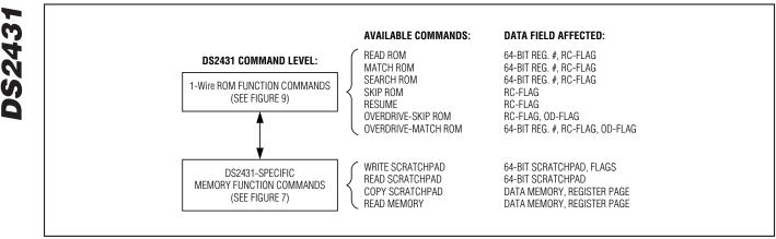
Figure 2. Hierarchical Structure for 1-Wire Protocol
