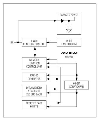
Figure 1. Block Diagram
