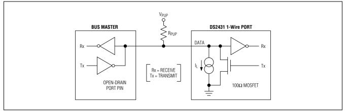
Figure 8. Hardware Configuration
